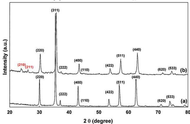
Figure 3. X-ray diffraction patterns of commercial powders (a) magnetite (Fe<sub>3</sub>O<sub>4</sub>), Sigma–Aldrich 310069 (b) maghemite (γ-Fe<sub>2</sub>O<sub>3</sub>), Sigma–Aldrich 544884. The characteristic (210) and (211) peaks of the maghemite phase are obvious.
