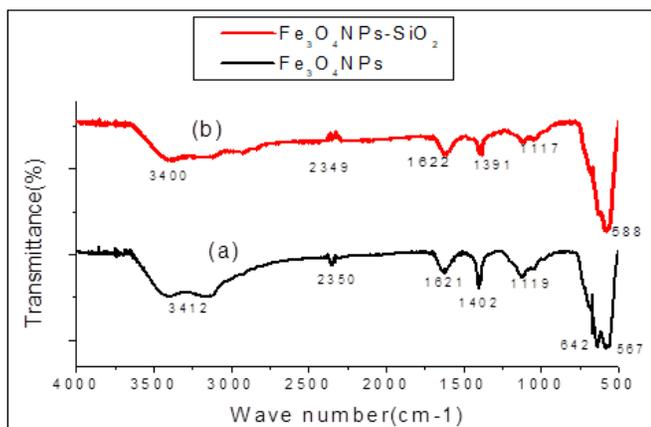
Figure 4: FT-IR spectra of (a) iron oxide NPs and (b) iron oxide NPs-SiO<sub>2</sub>.
