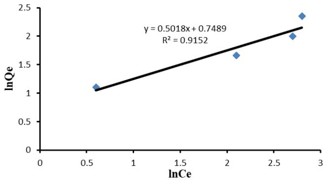
Figure 10: Linearized Freundlich isotherm (pH = 3, iron oxide NPs-SiO<sub>2</sub>= 0.7 g, room temperature).
