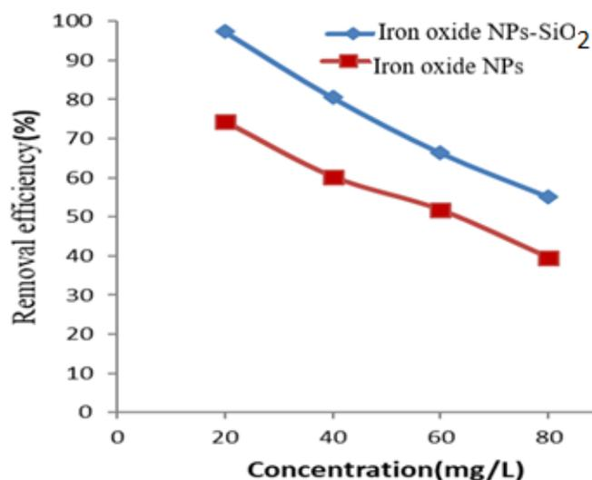
Figure 5. Effect of initial concentration of Cr (VI) on removal efficiency of iron oxide NPs and iron oxide NPs-SiO<sub>2</sub> (C<sub>0</sub> = 10–100 mg l<sup>-1</sup>, pH = 3, adsorbent dose = 0.7 g l<sup>-1</sup>, contact time = 120 minutes and room temperature).
