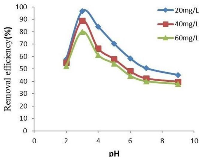
Figure 6: Effect of initial pH on removal efficiency by iron oxide NPs- $\text{SiO}_2$  ( $C_0 = 20, 40$  and  $60 \text{ mg l}^{-1}$ , adsorbent dose =  $0.7 \text{ g l}^{-1}$  and contact time = 120 minutes).
