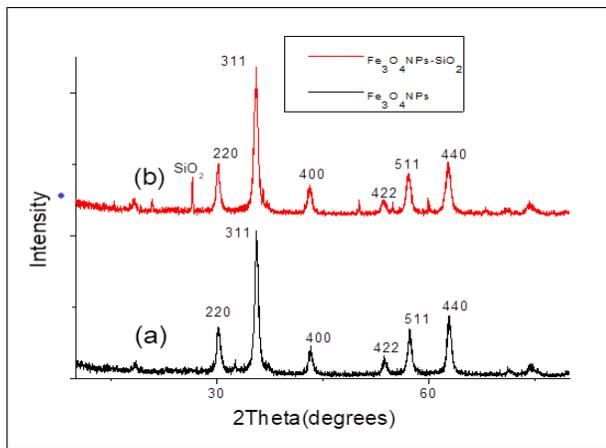
Figure 2: X-ray diffraction patterns of (a) iron oxide NPs and (b) iron oxide NPs-SiO<sub>2</sub>.
