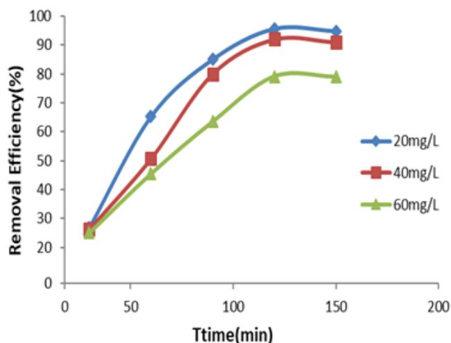
Figure 8: Effect of contact time on removal efficiency (C<sub>0</sub> = 20, 40 and 60 mg l<sup>-1</sup>, T = 25°C, adsorbent iron oxide NPs-SiO<sub>2</sub> dose = 0.7 g l<sup>-1</sup>, pH = 3, and room temperature).
