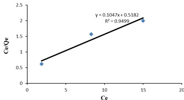
Figure 9: Linearization of the Langmuir isotherm (pH = 3, iron oxide NPs-SiO<sub>2</sub> = 0.7 g, room temperature).
