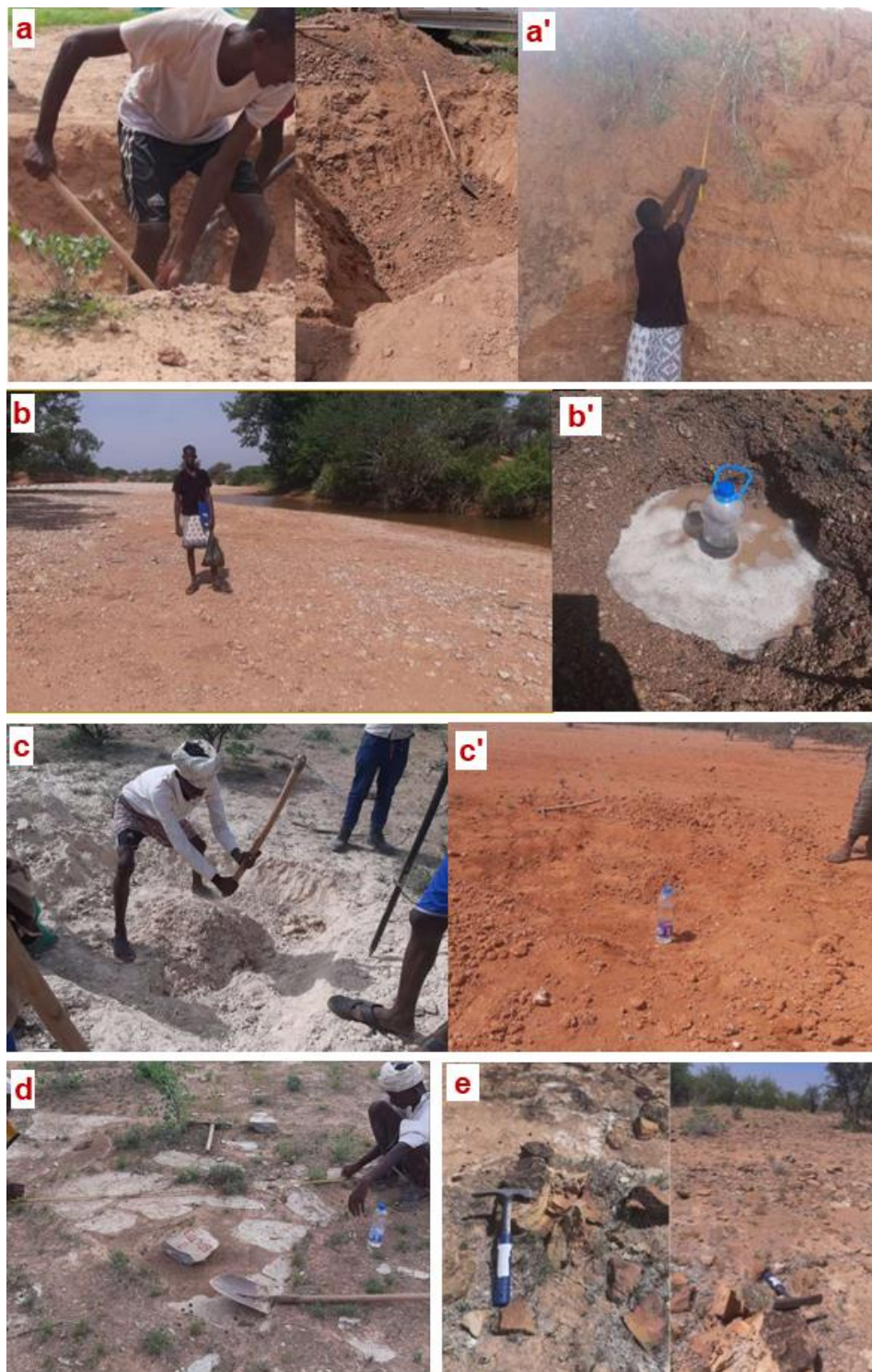
Figure 3: Photo showing the five geotechnical units identified: (a) Flood plain deposits (silty clay) at the RAS, a' Flood plain deposits at the LAS side of central valley; (b) channel deposit at the main dam central valley (sandy Gravel), b' Sand; (c) residual soil (completely weathered rock) at the RAS, c' residual soil at the center of the saddle axis; (d) gypsum rock mass at the LAS; (e) limestone/mudstone rock mass at the RAS upper margin
