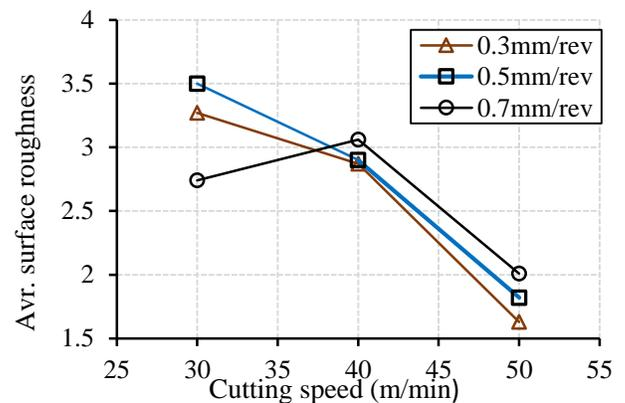
**Figure 6:** The effect of cutting speed on the surface roughness at 0.3 mm/rev feed, at 0.5 mm/rev and at 0.7 mm/rev.
