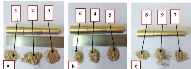
**Figure 7:** Chip morphology (a) for experiment 1, 2 and 3 (b) for experiment 4, 5 and 6 (c) for experiment 7, 8 and 9.
