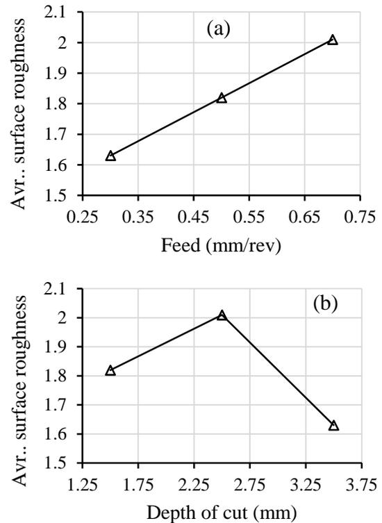
**Figure 5:** The effect of (a) feed and (b) depth of cut on surface roughness at cutting speed of 50 m/min.
