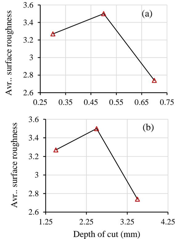
**Figure 3:** The effect of (a) feed and (b) depth of cut on surface roughness at cutting speed of 30 m/min
