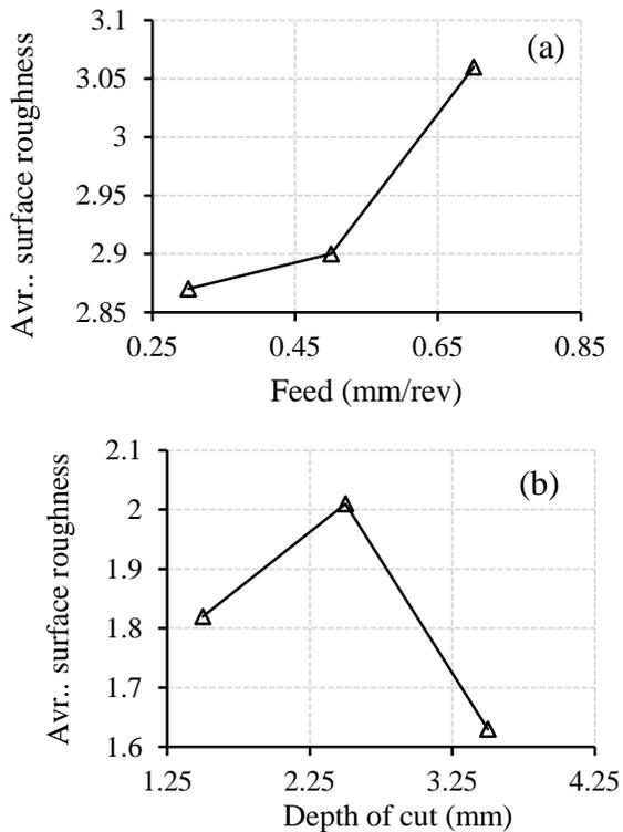
**Figure 4:** The effect of feed (a) and depth of cut (b) on surface roughness at cutting speed of 40m/min.
