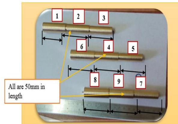
**Figure 2:** Samples after turning process
