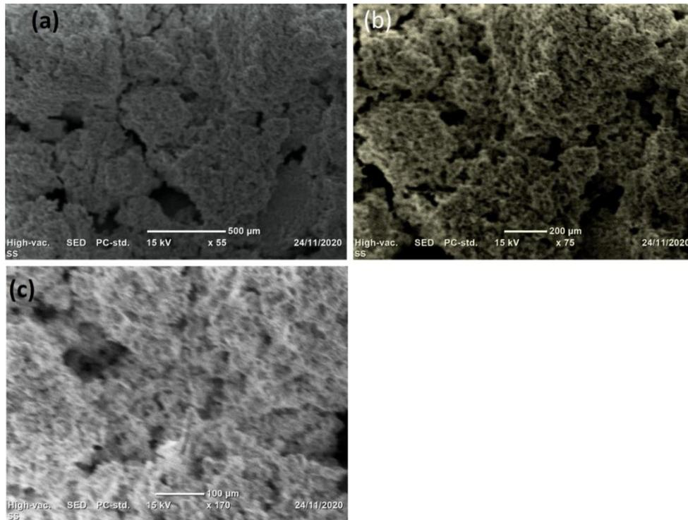
**Figure 3:** The SEM images of silica micro particles in different resolution of (a) 500 μm, (b) 200 μm, and (c) 100 μm.
