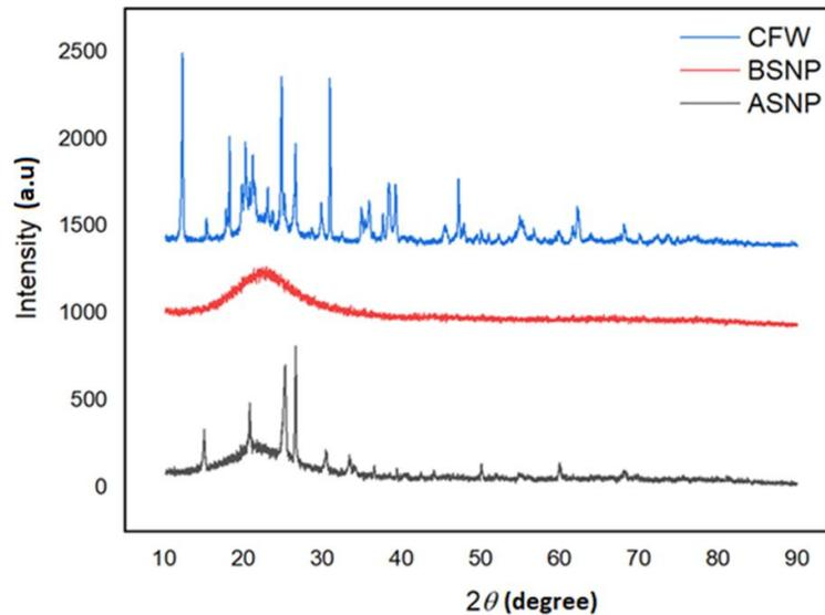
**Figure 4:** XRD analysis of three samples, chemical factory waste (CFW), basic step silica microparticles (BSNP) and acidic step silica microparticles (ASNP).
