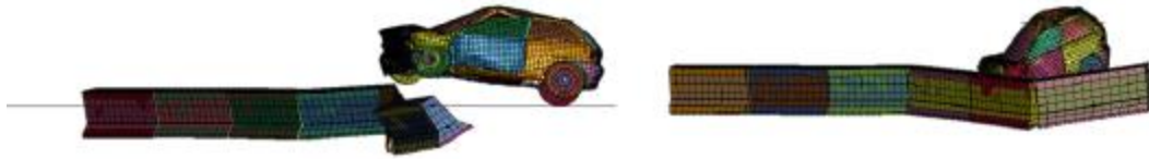
Figure 16: Vehicle swing slide at large collision angle
