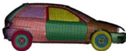
Figure 5: Mesh generation for the whole vehicle
