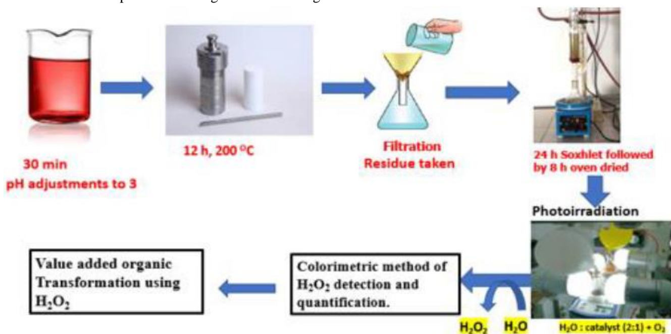
Figure 2: The overall design of experiment and synthetic scheme (catalysis and post catalysis)
