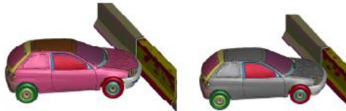
Figure 8: Vehicle crash configuration at large collision angle
