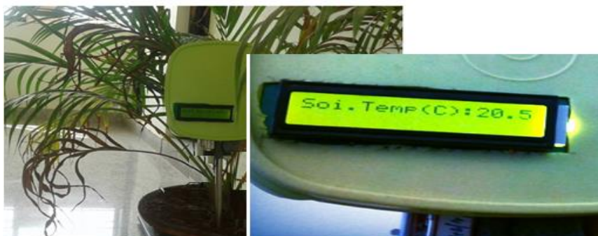
Figure 14: Application of the fabricated thermometer in real-time soil temperature monitoring in agriculture
