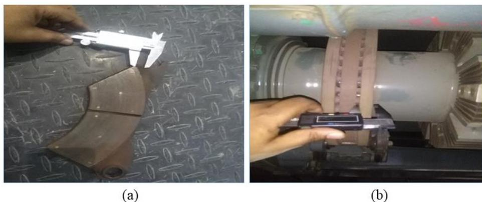
Fig. 2 Disc and pad dimensional data extractions at AALRT (a) pad (b) disc
