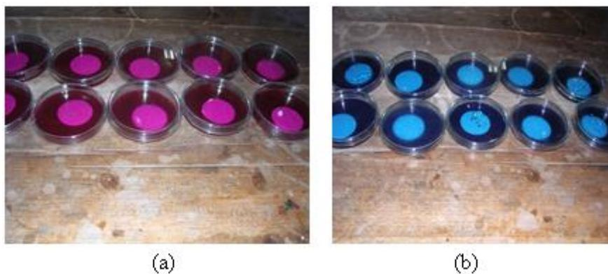
Fig. 4. Total coliform colonies in membrane filtration (a) and Faecal coliform colonies in membrane filtration (b)
