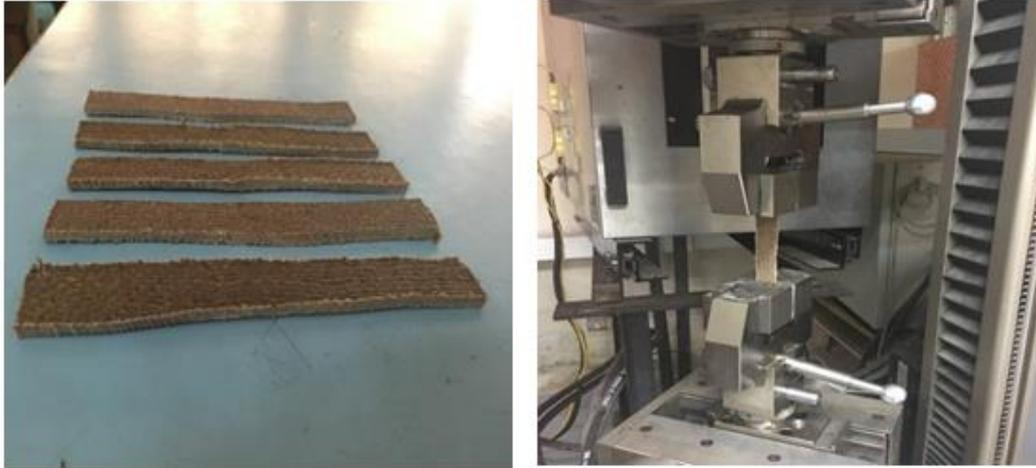
Fig. 3 Specimen preparation and testing on Zwick composite tensile testing machine
