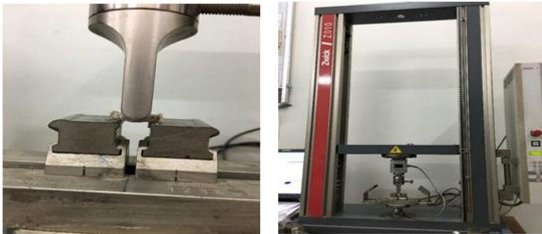
Fig 4 Specimen testing on Zwick/Z010 shear strength tester
