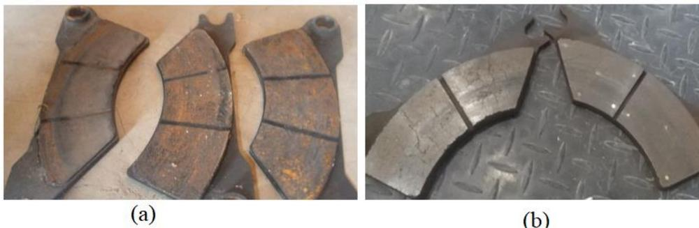
Fig. 4 Damaged friction surface due to thermal stress: (a) two radial grooves, (b) one radial groove, (camera view from AALRT)
