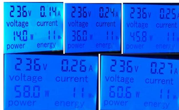
Fig. 16 Power consumption of composite fan blades (six fabric layers & 50% Volume fraction) at different speeds and pitch angle of 10.13<sup>0</sup>
