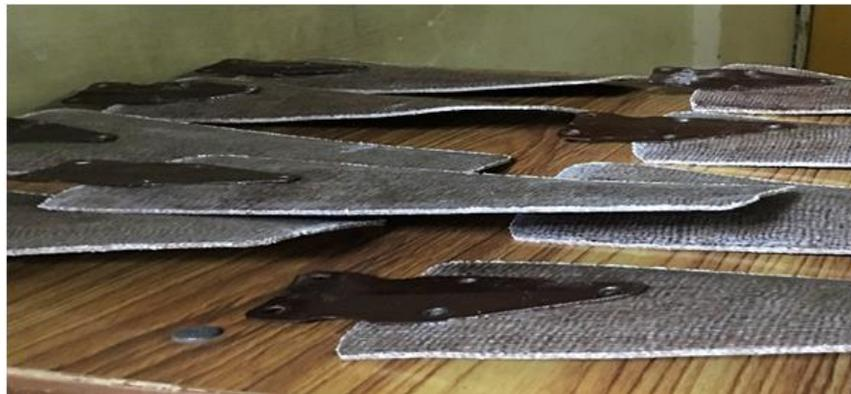
Fig 18 Jute-PLA composite blades made with different pitch angles
