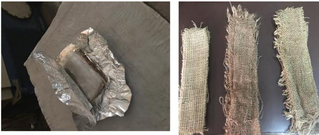
Fig. 2 Jute fabric layer and PLA film stacking for making composite blade
