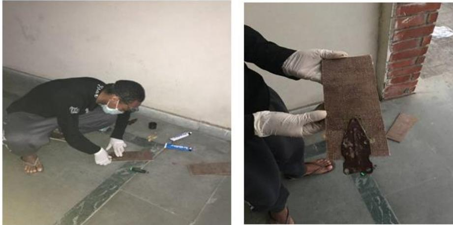
Fig 17 Joining of the metal plate with the composite blades using Araldite epoxy
