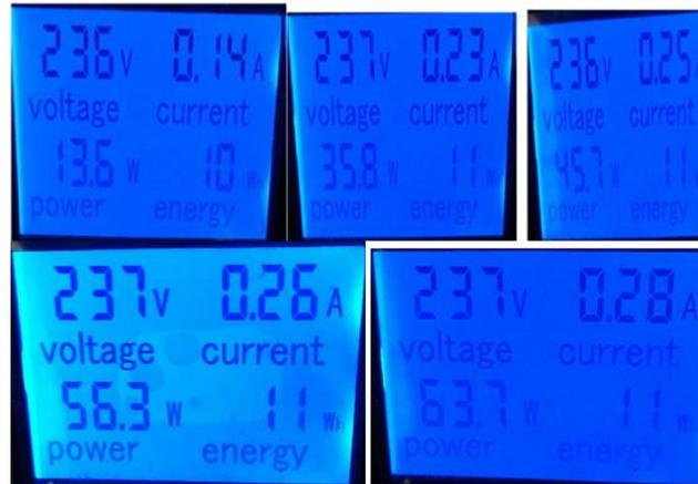
Fig. 15 power consumption of composite fan blades (six fabric layers & 50 % Volume fraction) at different speeds and pitch angle of 12<sup>0</sup>
